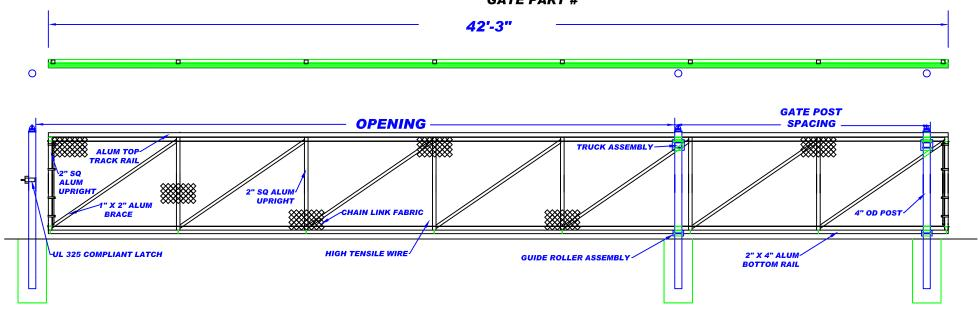
GATE ELEVATION - SHOWN OSLI, OPENS TO RIGHT UNIVERSAL DESIGN (CAN BE INSTALLED TO OPEN LEFT  $\ \underline{OR}\ RIGHT)$
