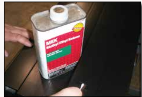
PCI#8 Solvent Cure Test Solvent testing per PCI#8 is completed hourly to test for complete cure.
