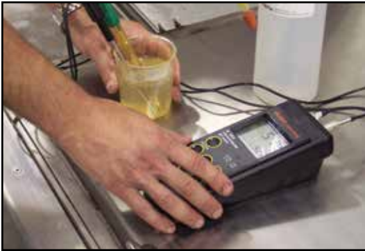
System Titration Test The pH levels are checked twice per shift as part of the pretreatment titration check.
